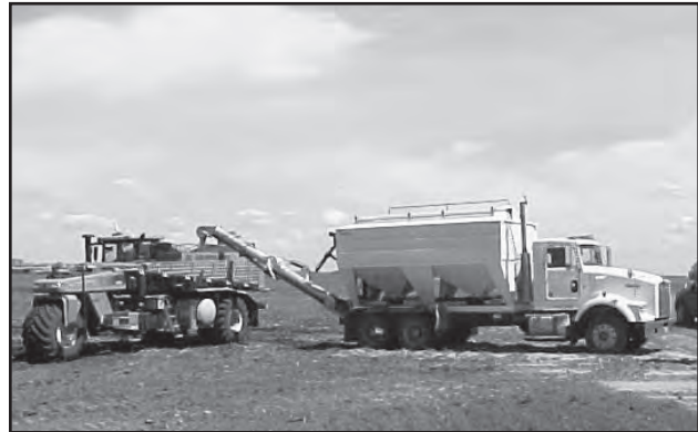
Fig 24 - Unloading into Floater
